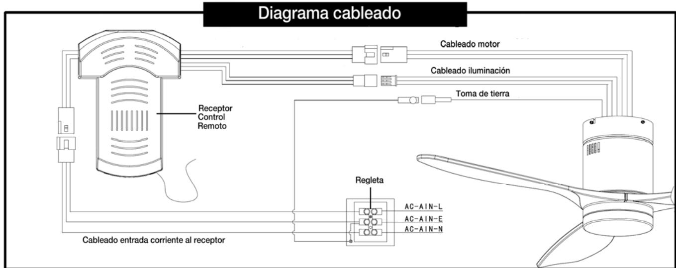
2 - Connect the power cables to the terminal strip connector.
